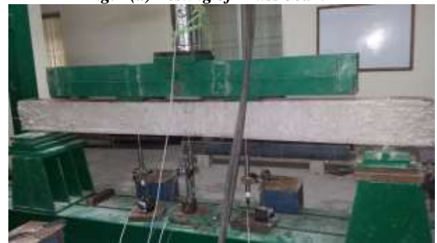
Fig. 2(b) Testing of Composite beam
