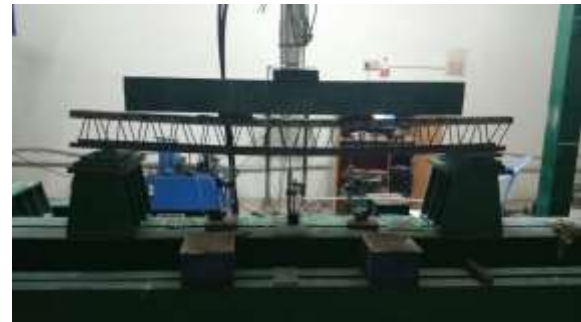
Fig. 16 Truss beam failure
