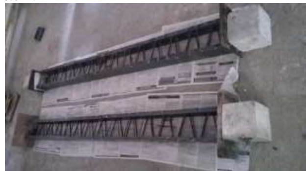
Fig.1(a) Fabricated Truss beams
