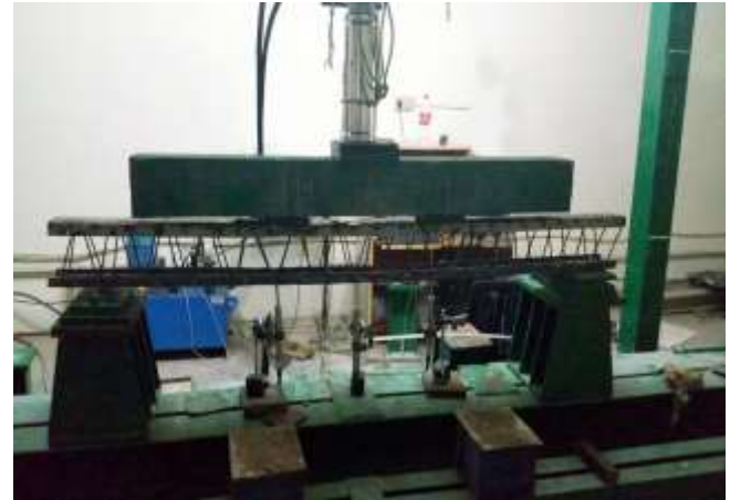
Fig. 2(a) Testing of Truss beam
