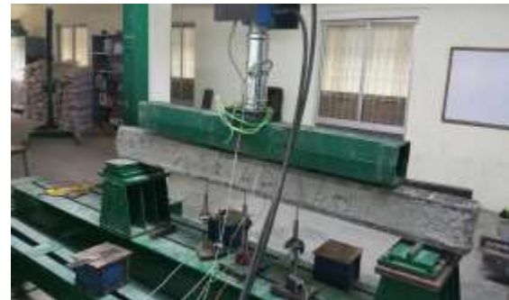
Fig. 16 Composite beam failure
